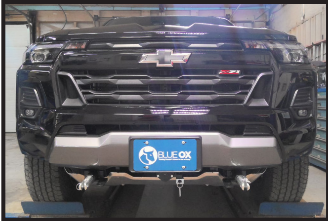
10a. Chevy Colorado Models: Reinstall the belly pan, skid plate, fascia, and reconnect all electrical connections.
