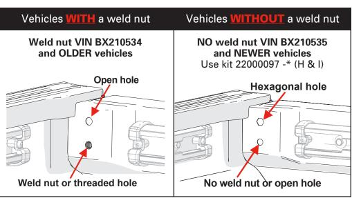
If you have a vehicle WITH a weld nut, VIN BX210534, and OLDER vehicles. Install the cab brackets (B & C) by inserting the hex button head screw with washer (E) through the upper hole of the cab brackets (B & C). Then install the M8 bolt T-50 (D) through the bottom hole in the cab brackets (B & C). On the backside of the bracket (B & C) thread a washer (F) and a well nut (G) onto the bolt (D).
