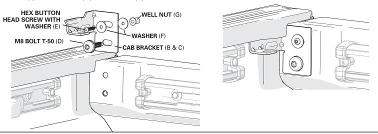
If you have a vehicle WITHOUT a weld nut, VIN BX210535, and NEWER vehicles. Place the bulkhead brackets (H) underneath the truck's bed flange and align with the 2 holes in the bulkhead. Install the cab brackets (B & C) by inserting the M8 bolt T-45 (I) through the upper hole of the cab brackets (B & C). Then install the M8 bolt T-50 (D) through the bottom hole in the cab brackets (B & C). Make sure that both fasteners go into the bulkhead brackets (H).
